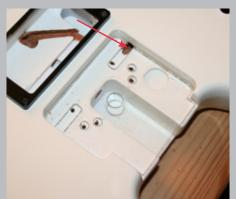
This hole directly leads into the control cavity. Make sure you've got the right angle (not too steep), otherwise the hole ends outside the cavity.
