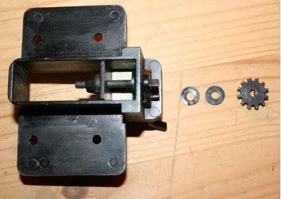
There should be another thin washer between the lever and the trem base. You can leave it where it is, just make sure it's correctly placed when installing the new spring tension adjuster.
