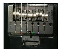
This is the documentation of my (successful) attempt to find a fix the tremolo system, which obviously is faulty by design, caused by weak pedestals for the hinge posts.
