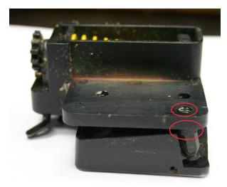
After removing the base plate the problem is clearly visible: In most cases not the two posts are bent, but the short pedestals on the base plate. This could also be caused by the posts, because their threaded ends are too short, so they are only held in the upper part of the pedestal. They don't reach the lower end of the thread. Since the threaded ends of the posts were too short, all the tension of the strings was held by the two pedestals only.
