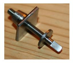
Another weak point is the spring tension adjuster. This is a plate sitting on a threaded rod, compressing the spring in the trem. The compression must be adjustable to set a perfect balance between the string tension (pulling the trem up) and the force of the spring (pushing the trem down). A perfectly balanced setup makes sure that the trem has exactly the same position in locked and unlocked state.
