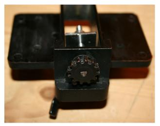
Reinstall the washers and the cog. Tighten the grub screw again to fix the cog on the rod.
