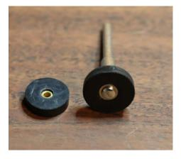
Hold the saddles **tightly** when burnishing the rollers, or clamp them in a vise. Burnish them for a few seconds at high speed (25.000-30.000 rpm). The tool rotating at high speed is quite powerful, so make sure you have a tight grip on the saddle.
