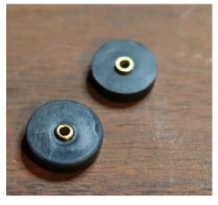
With a washer above and below the hole (I've used the same washers as used on the TT bearing pins) screw the rubber tap washer onto the mandrel. Tighten as needed, the little ball end inside will prevent the rubber from getting compressed too much.
